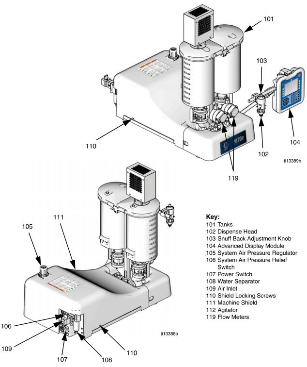
Fig. 1:PR70v with On-Board Tanks and Other Options
